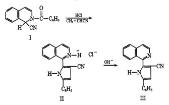
Brief treatment of III with hot 80% sulfuric acid resulted in simultaneous sulfonation and hydrolysis of the compound, as indicated by the infrared spectrum and the elemental analysis of the product. The resulting 2-(1-isoquinolyl)-3-carboxamido-5-phenyl-4pyrrolesulfonic acid (IV) was isolated in the form of its sodium salt. This acid, by further treatment with dilute sulfuric acid, was converted to the diacid V, which was isolated in the form of the disodium salt.
